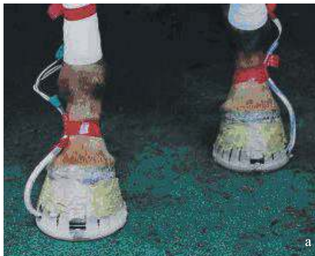
Figuur 3. a) Geïnstrumenteerde hoefijzers b) dwarsdoorsnede van deze zogenaamde 'force shoes' (uit: AJVR, 2000, 61: 980-981, Kai et al. "Use of an instrument sandwiched between the hoof and shoe to measure vertical ground reaction forces and three-dimensional acceleration at the walk, trot, and canter in horses").
