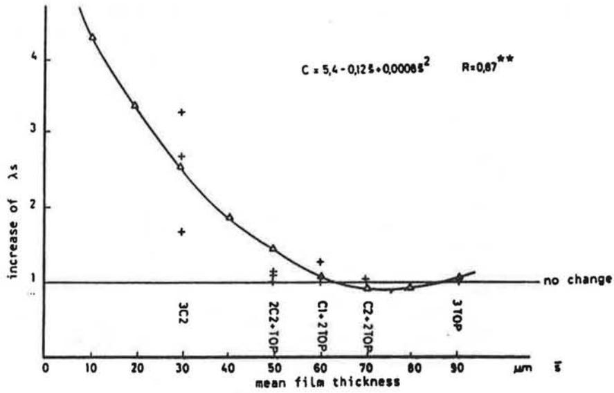
FIGURE 4: Determination of the critical film thickness  $s$ .
