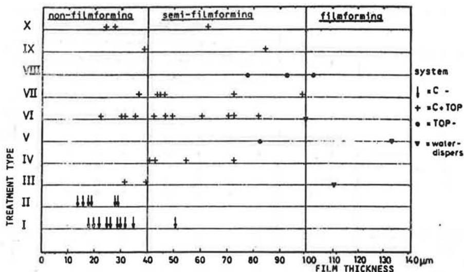
FIGURE 2: Penetration values obtained according to the DIN52162 standard compared with the Biological Effective Penetration Depth.
