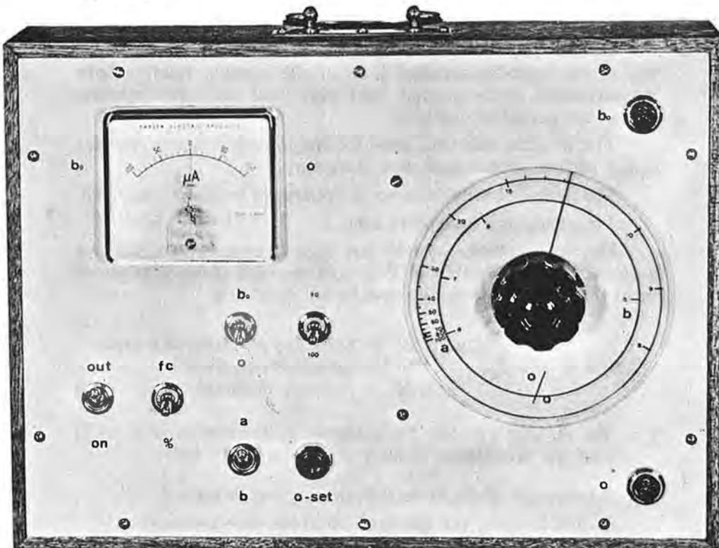
Photo 1. The operational part of the relative light intensity meter with compensating circuit.
