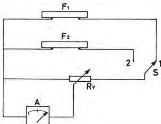
Fig. 1. The principle of the relative light intensity meter constructed by Brechtel 1962.
