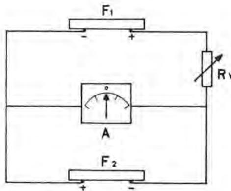
Fig. 2. The principle of a relative light intensity meter with compensating circuit.
