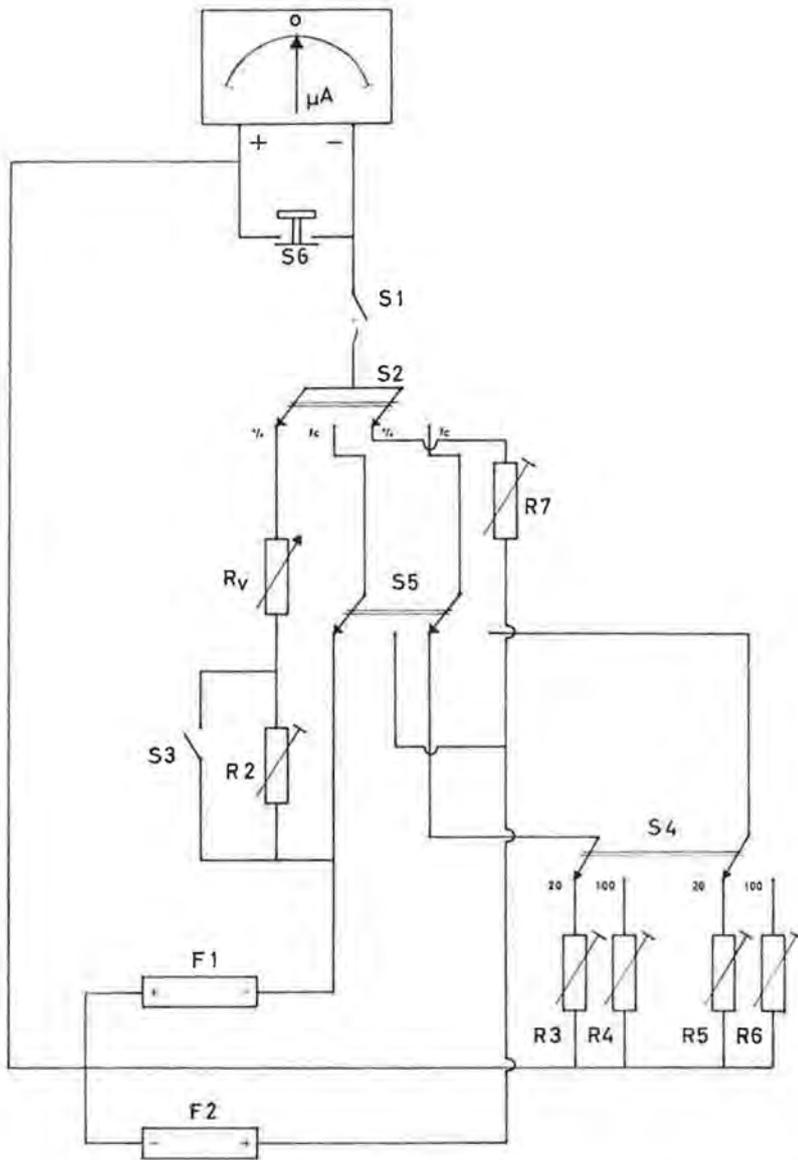
Fig. 4. The practical outline of the relative light intensity meter with compensating circuit and with possibilities for absolute measurements.
