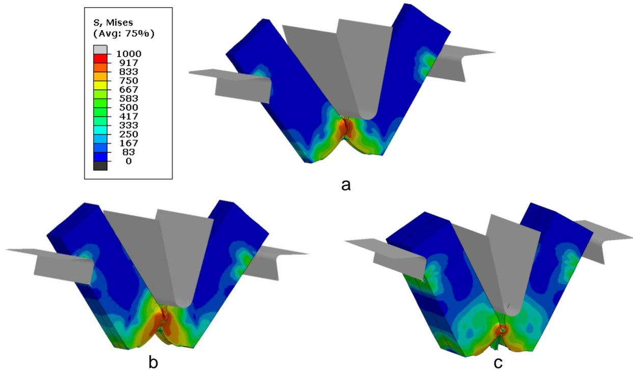
Figure 5: FEA results (von Mises stress) of CVN specimens with thickness of a) 2.5 mm, b) 5.0 mm and c) 10 mm.
