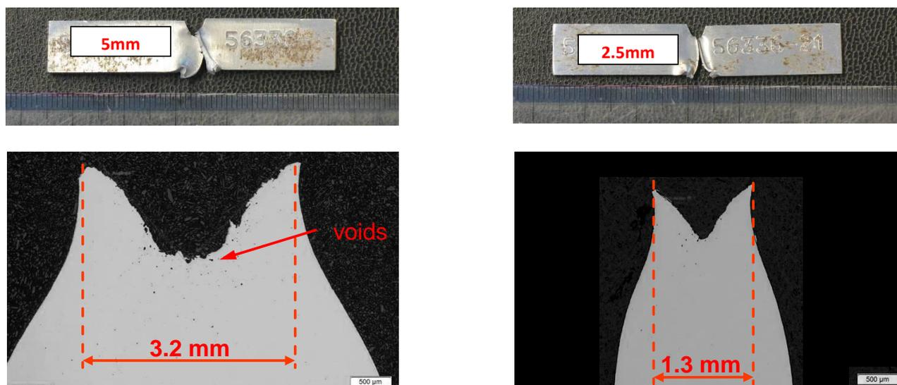
Figure 2: Reduced thickness CVN specimens after impact testing. The bottom pictures show a section view of the slanted fracture surface with two shear lips.
