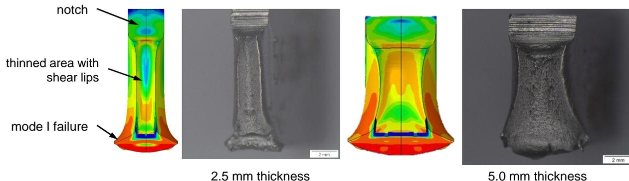
Figure 7: Comparison between modelled and experimentally obtained fracture surfaces.
