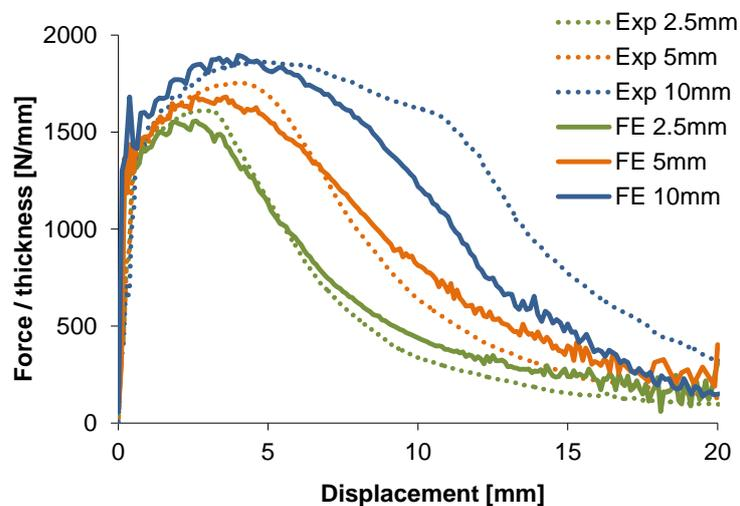
Figure 6: Comparison between modelled and measured force-displacement curves.
