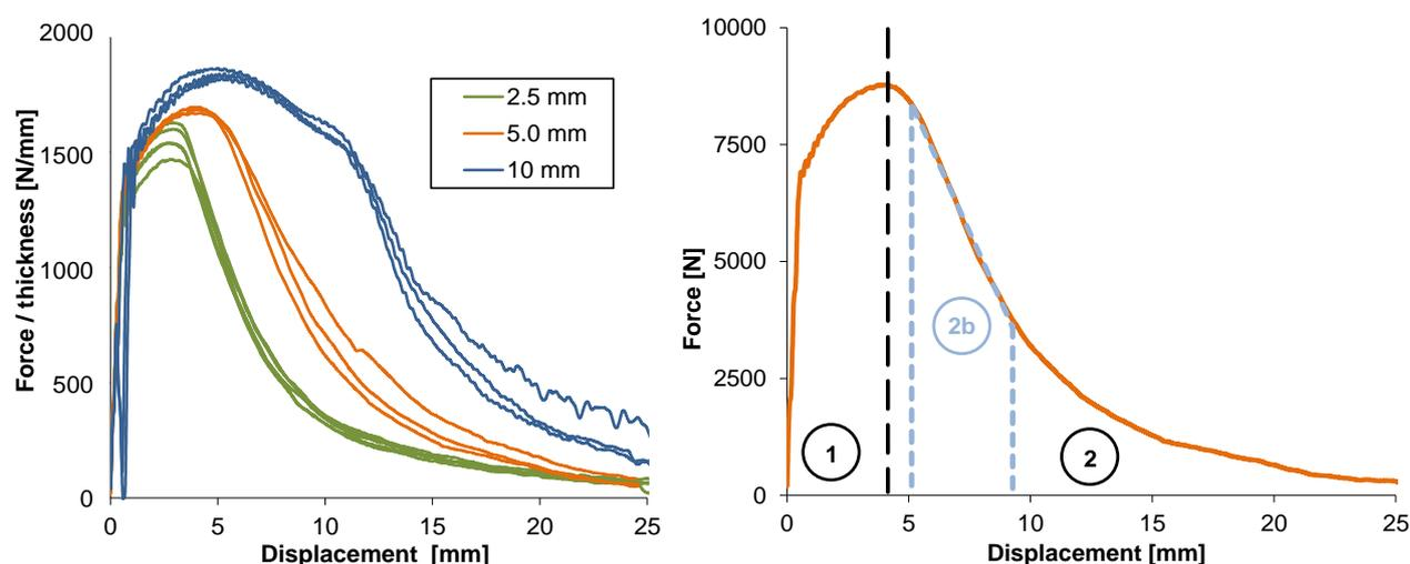
Figure 3: Left: Normalised force-displacement curves for CVN samples of 2.5 mm, 5.0 mm and 10 mm thickness at room temperature. Right: Force-displacement curve from instrumented CVN experiment on an X70 sample with a thickness of 5 mm at room temperature (fully ductile failure). Areas 1 and 2 are respectively the crack initiation and propagation regions. Area 2b is the region of linear crack propagation.
