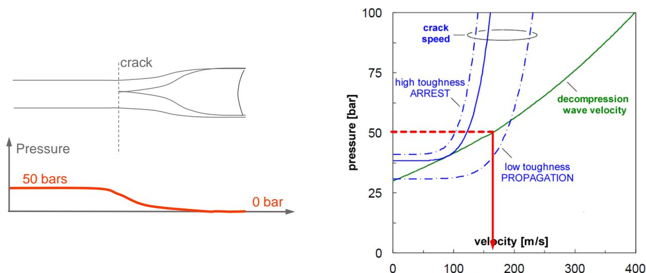
Figure 1: left: pressure evolution during longitudinal crack propagation; right: Battelle Two Curve Method [2].
