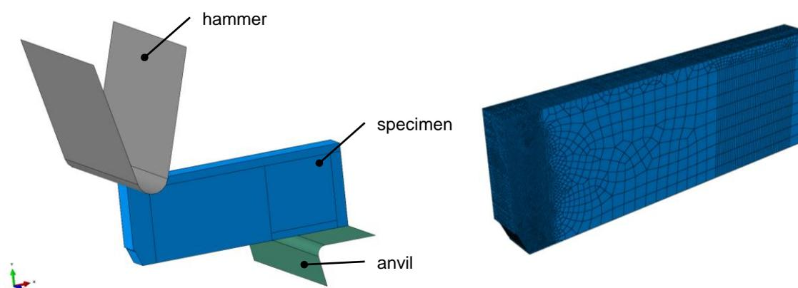
Figure 4: left: parts of FEA model; right: mesh ¼ of CVN specimen.
