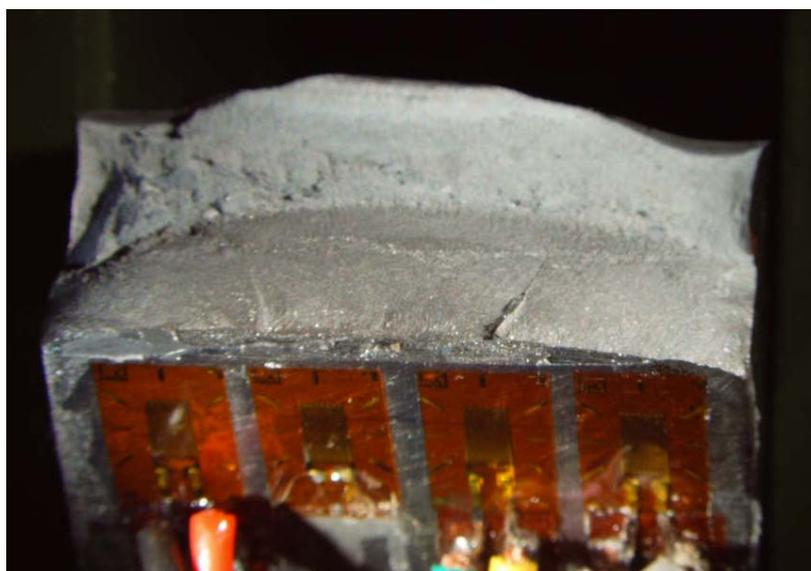
Figure 12: Cross section of fractured specimen and location of strain gage sensors, magnification x5
