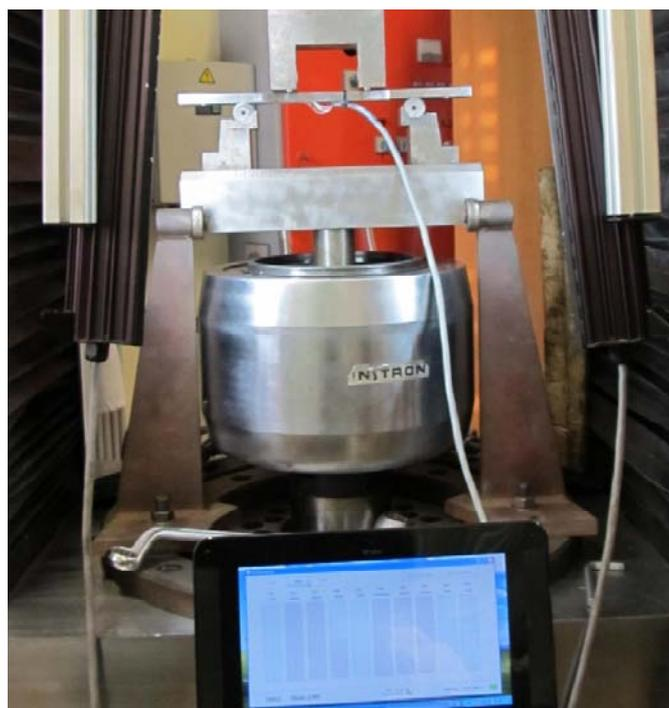
Figure 6: Four point bending fatigue testing of specimen with multiple strain gauges with Dynastrain device
