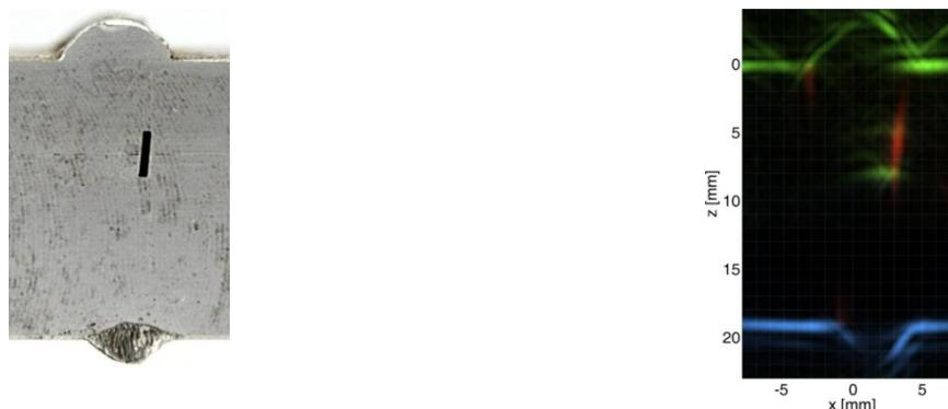
Figure 2 Metal cross section and IWEX image of an artificial flaw showing accurate representation of the size and orientation of the flaw. Also note the green signals at the tips of flaw which are used for sizing purposes. The capability can be used to determine the flaw type.
