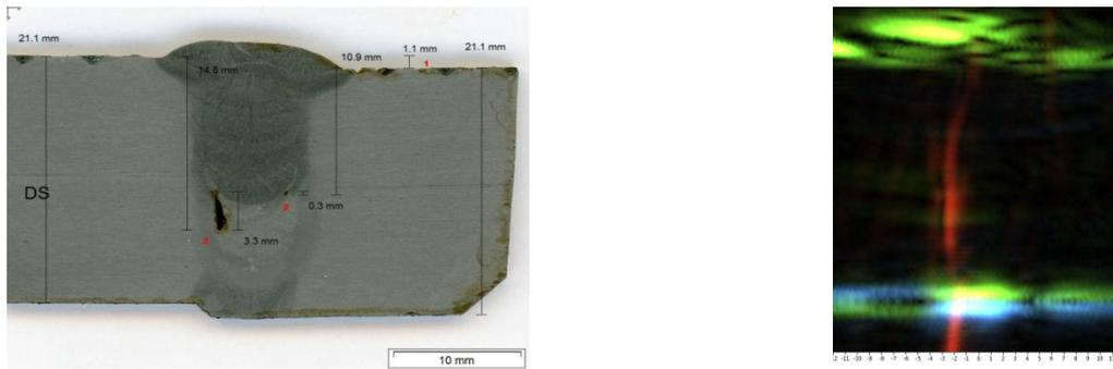
Figure 3 Macro sectioning and IWEX image of a weld showing a defect and high-low. The presence of high low in the image is clearly indicated by the green and blue signals on the ID. Notice how green, the ultrasonic signal coming from the left, and blue, the ultrasonic signal from the right, are flipped at weld centre
