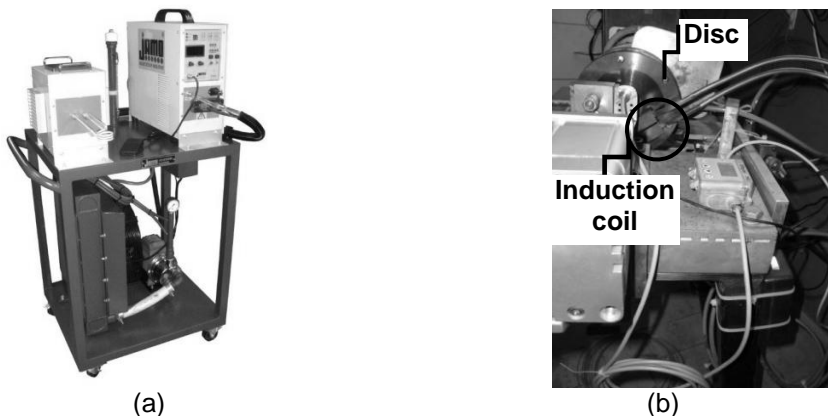
Figure 2. Induction heater integrated to the tribometer: (a) induction heater equipment and (b) detail of the induction coil installed 1 mm close of the disc surface
