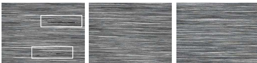
Figure 5. Defects after 50 crash simulations on air bearing (Type 3) and beam surface
