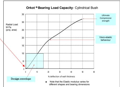
Figure 3 Typical load/ deflection curve of Orkot<sup>®</sup> composite, Trelleborg Product Information- Hydro Engineering Manual
