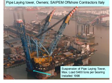
Image; Pipe laying tower, 135 metres tall with a deadweight 2400 tons, added in 1998 to the existing crane barge to enhance it's operational capabilities in offshore construction and pipe laying. The bearings passed their 10-year examination in 2008 and were declared 'fit for purpose'.
