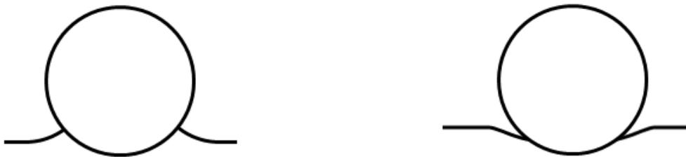
Figure 4: Pile-up (Left) and sink-in (right) influences the accuracy of stress and strain calculations
