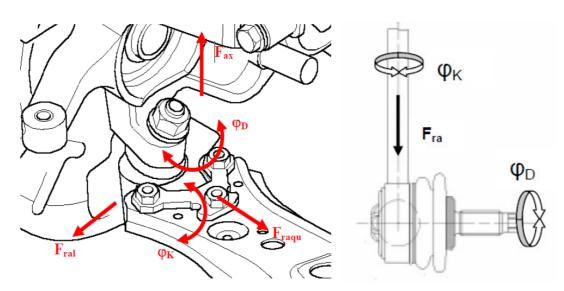
Figure 3: rotational and tilting movements of a ball joint in an automotive example [2]
