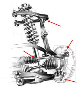
Figure 1: Toyota FJ Cruiser front suspension [1]
