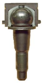
Figure 2: Cutaway section of a ball joint
