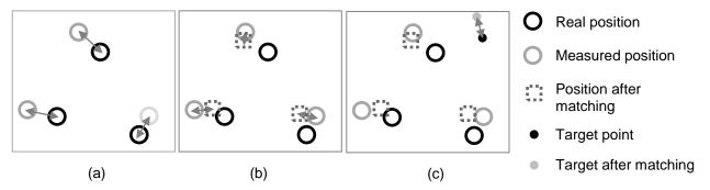
Figure 2: kind of errors for an optical tracking system: (a) FLE for each fiducial. (b) FRE at the fiducial positions after the matching procedure. (c) TRE at the target after the matching procedure.
