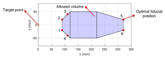
Figure 9: Allowed space and optimal solution for the fiducials for a 2D configuration
