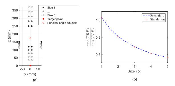
Figure 6: Widespread of the z-coordinate of the fiducials, with constant center of the fiducial cloud. (a) Sketch of the configuration for size 1 to size 5. (b) TRE divided by FLE for the different sizes. Formula 1 is plotted as well as the simulation (red dots).
