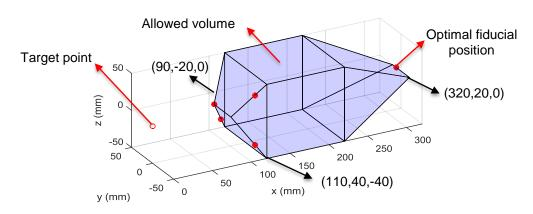
Figure 8: Allowed volume and optimal solution for the fiducials when a 3D configuration is used.
