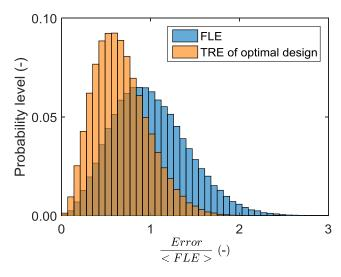
Figure 10: FLE and TRE distributions of the optimal design
