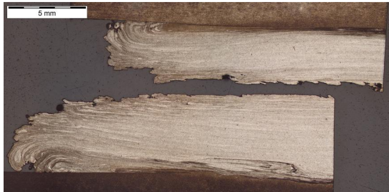
Fig. 9: Typical macrograph of an etched cross-section.
