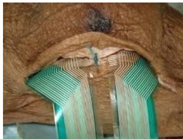
Figure 3. Positioning of the pressure film sensor.
