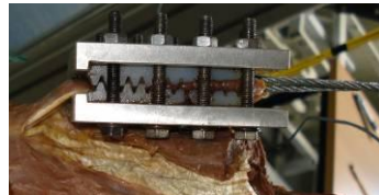
Figure 1. The clamping system for the rectus femoris and vastus intermedius
