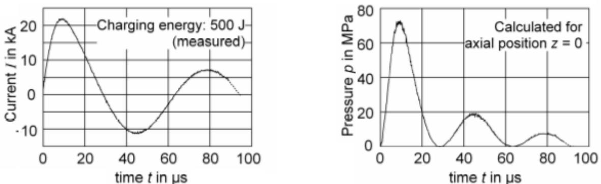
Figure 3: Discharge current and magnetic pressure [9]
