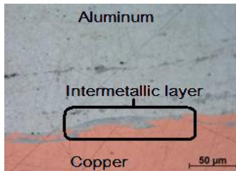
Figure 5: Microscopic image of a copper-aluminium MPW weld
