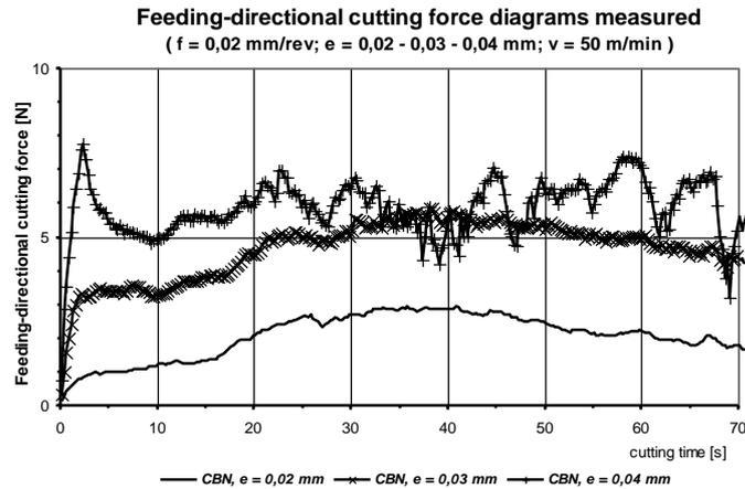
Figure 9. Diagrams of force in feeding direction.
