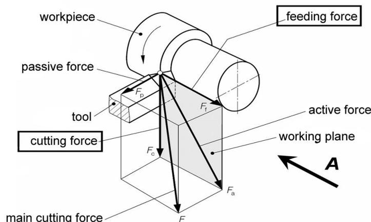
Figure 2. Cutting force components (ISO 3002/4, DIN 6584).
