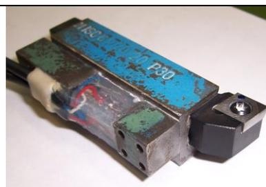
Figure 4. The photograph of the measuring tool-head finished with the holder clamped.
