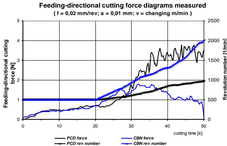
Figure 7. Diagram of cutting force in feeding direction.
