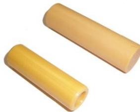
Figure 1. The zirconium-dioxide (Zn40)ceramics used at tests.
