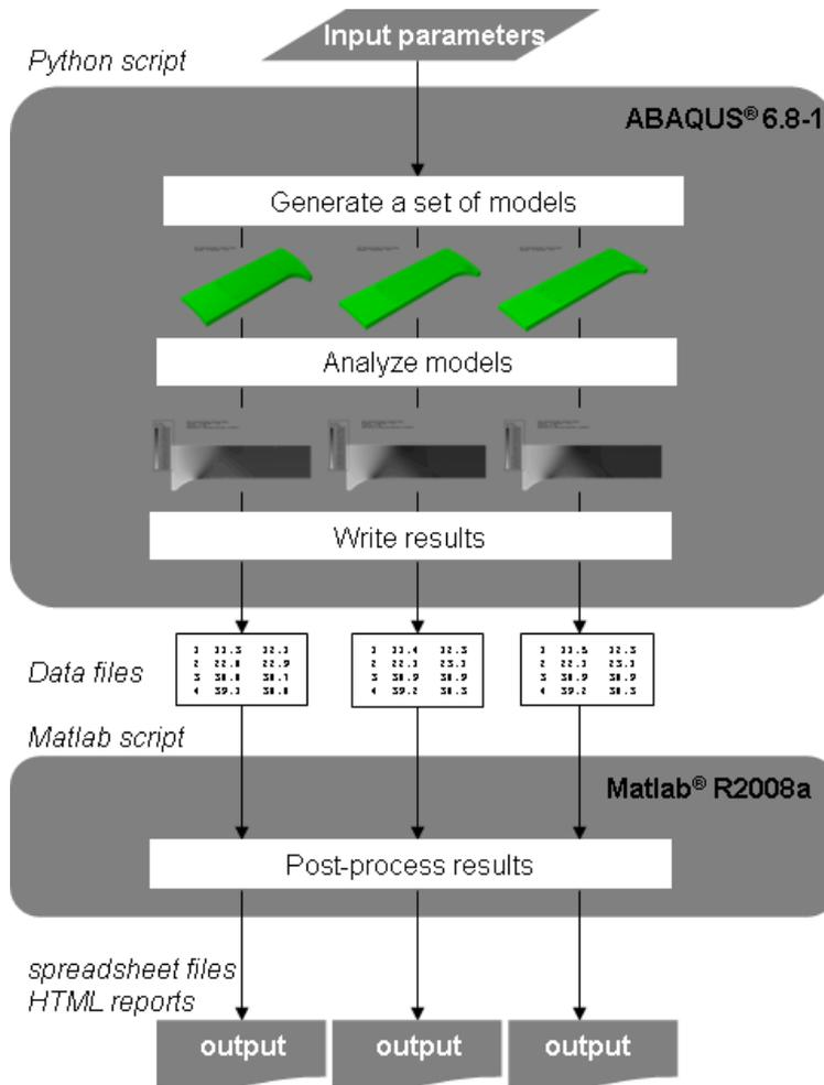
Figure 4: Structure of a parametric finite element study [22].
