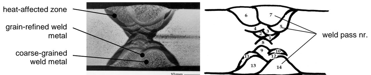
Figure 7: Heterogeneity in and around a weld metal, due to subsequent thermal cycles for each weld pass [1].
