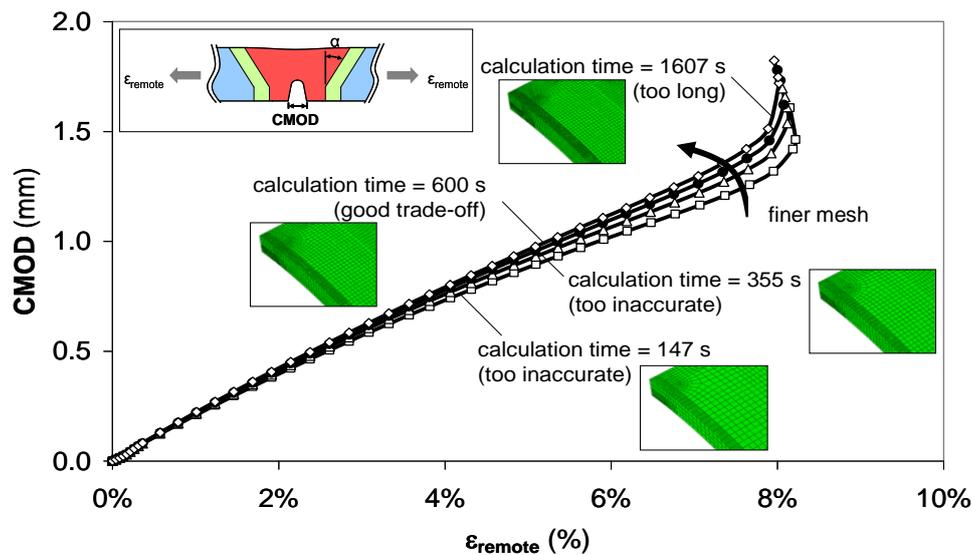
Figure 11: Example of a mesh convergence study.
