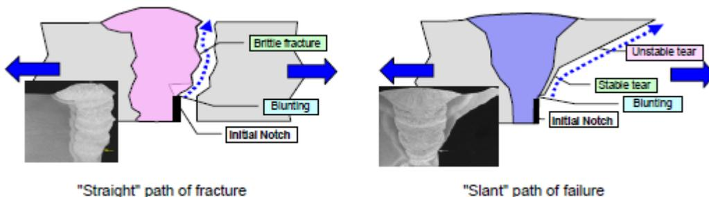
Figure 9: An initiated crack can grow in different directions, depending on the loading pattern and the local microstructures it encounters [24].
