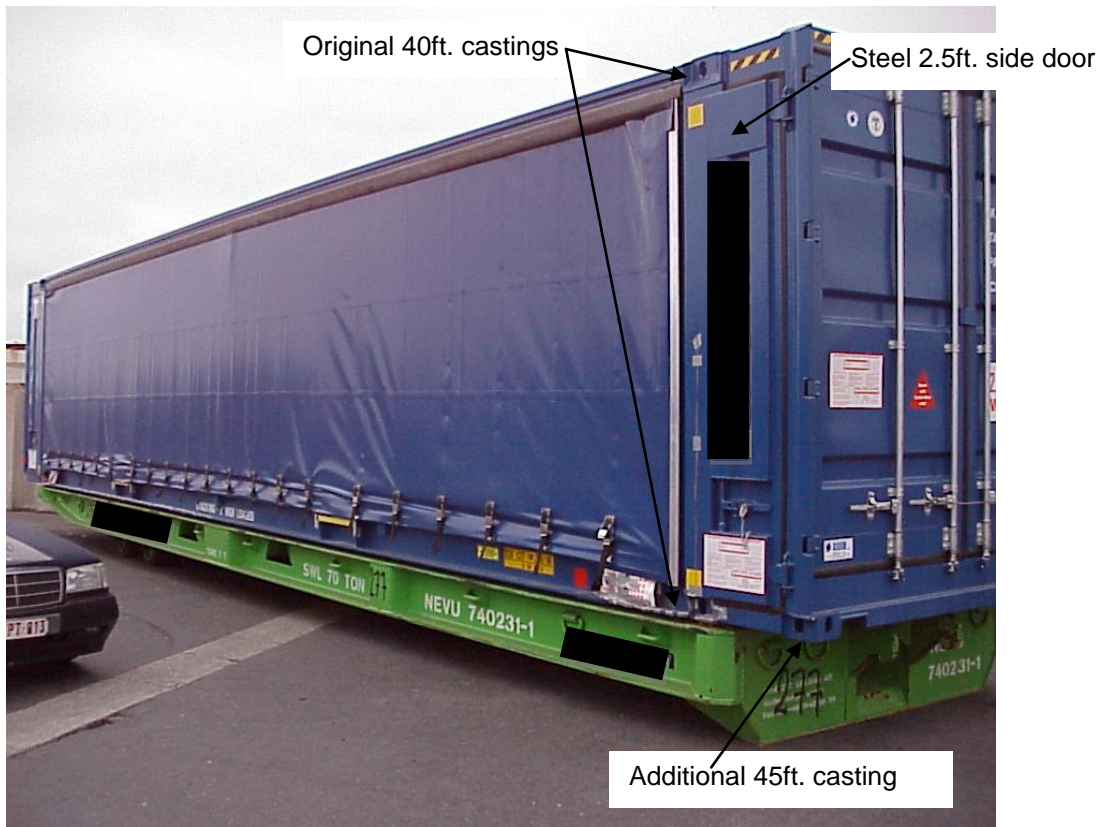
Figure 3. View from the back of a container of the same type on a 40ft. handling trailer
