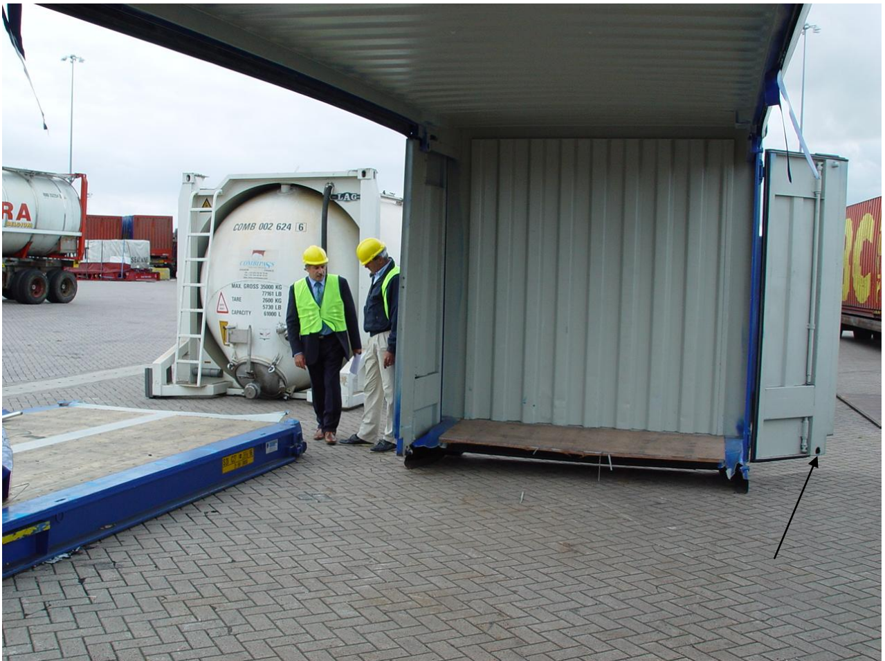
Figure 7. View of the front side of the container. Notice the bottom pin of the right hand side door is missing.
