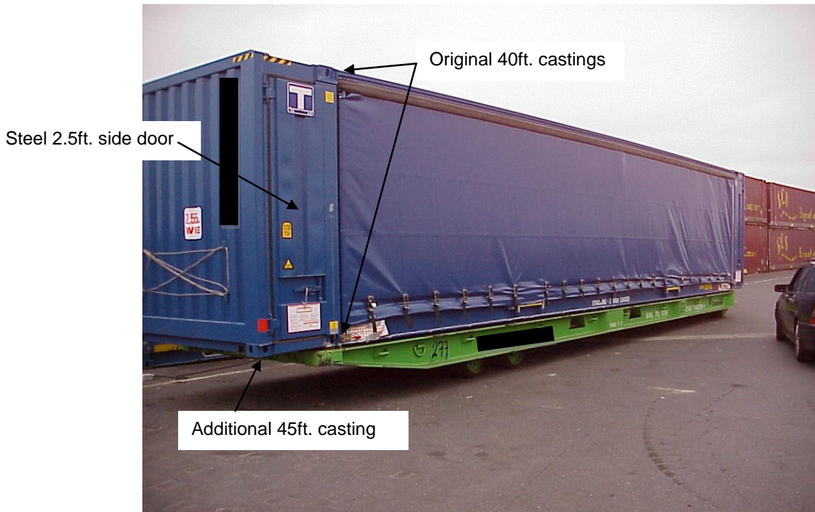
Figure 2. View from the front of a container of the same type, on a 40ft. handling trailer.
