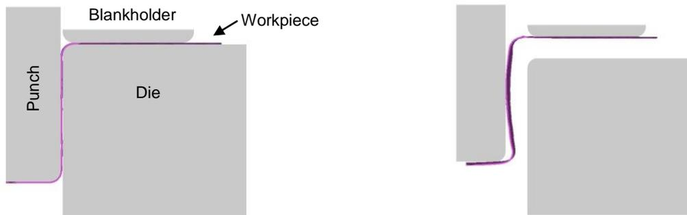
Figure 5. Position of die, punch, blank holder and workpiece before and after load releasing, left to right respectively
