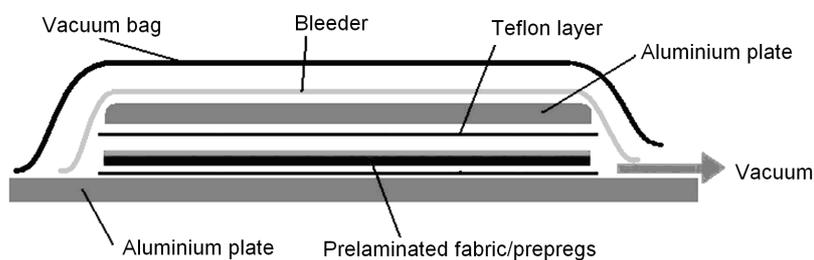
Figure 1. Carbon fibre reinforced epoxy's production set-up
