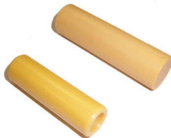
Figure 1. The zirconium-dioxide (Zn40) ceramics used at tests.
