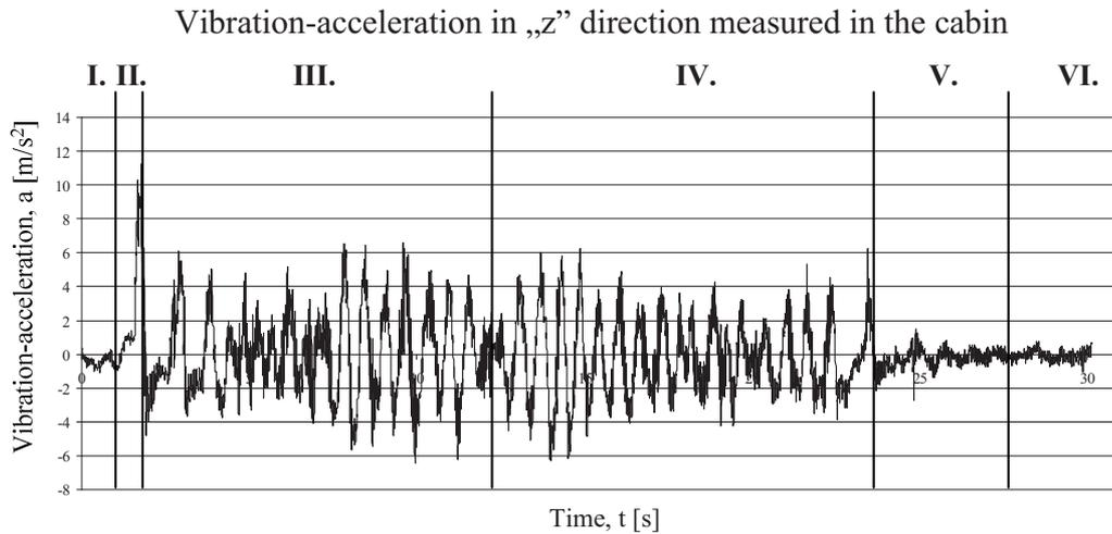
Figure 5. Characteristic sections of vibration-acceleration in „z” direction in the function of time measured in the cabin
