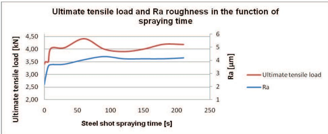
Figure 3. Effect of the steel shot spraying time
