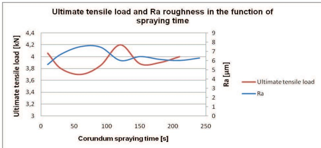
Figure 4. Effect of the corundum spraying time
