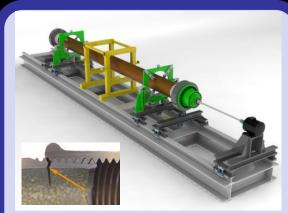
Fatigue testing and analysis. E.g. research on pipe joints in a full scale resonant bending fatigue setup.
