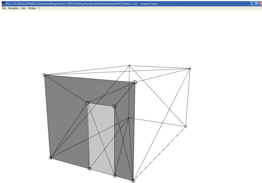
Figure 3 The closed and directed triangulated mesh, representing the internal geometry.
