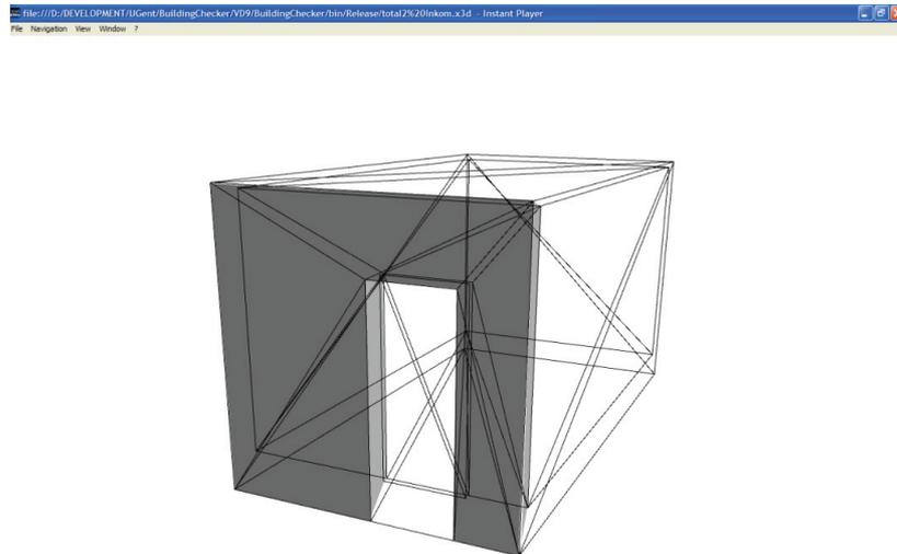
Figure 4 The inflated mesh, representing the external geometry for a lfcSpace instance.
