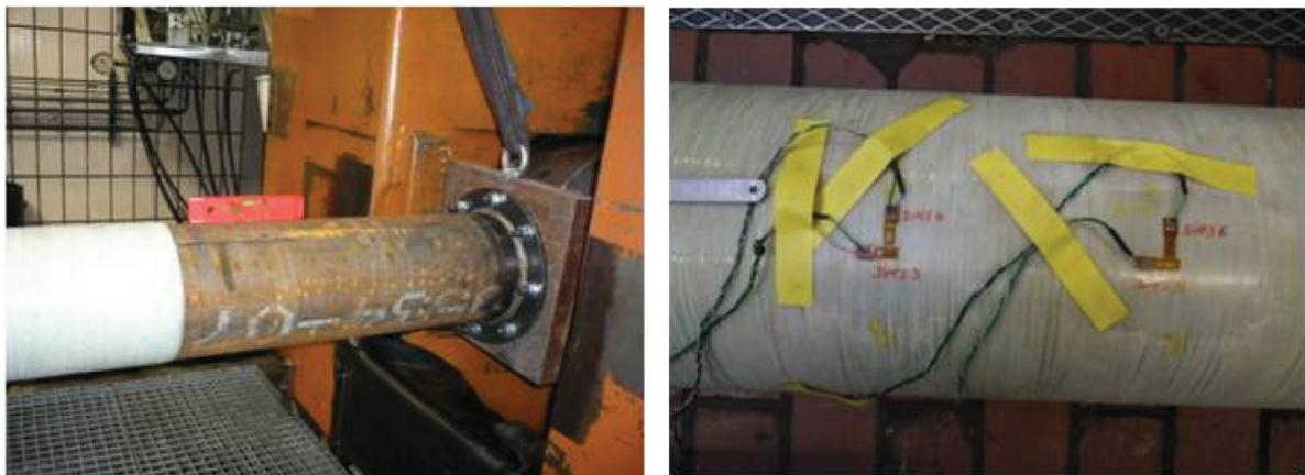
Figure 3: Clamping support (left) and strain gauge arrangement (right)
