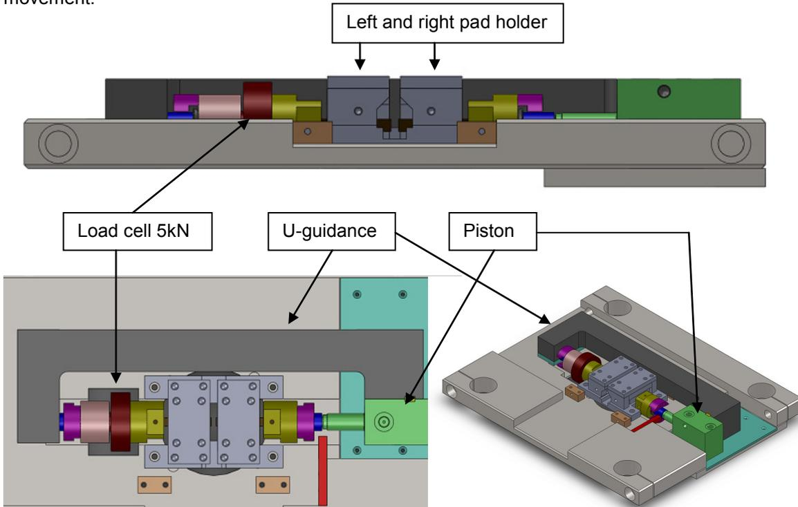
Figure 9: Concept 2: fretting fixture based on wedges
