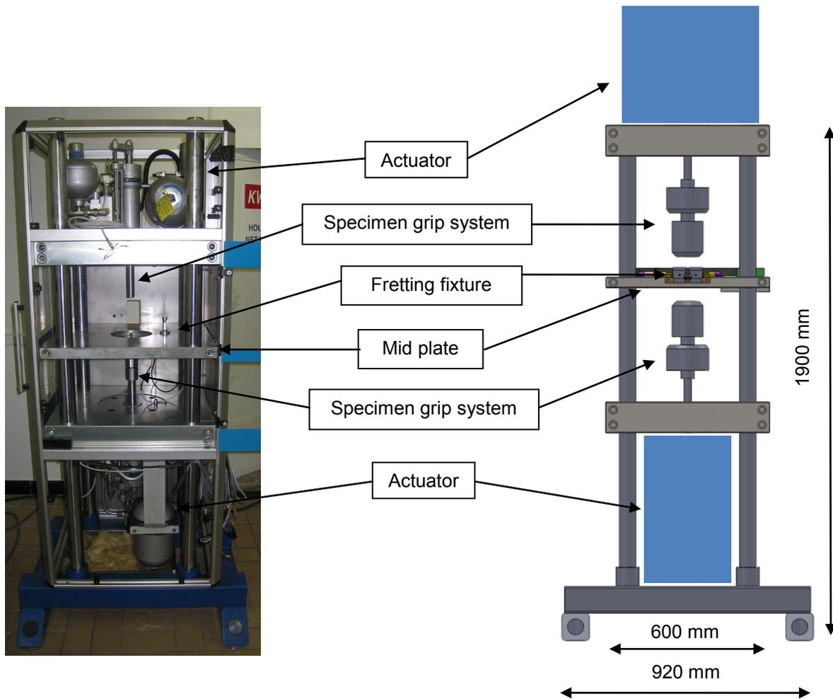
Figure 6: General view of the available machine and the future test fixture
