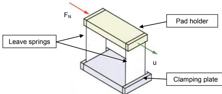
Figure 11: Fretting fixture based on a flexure mechanism [1]
