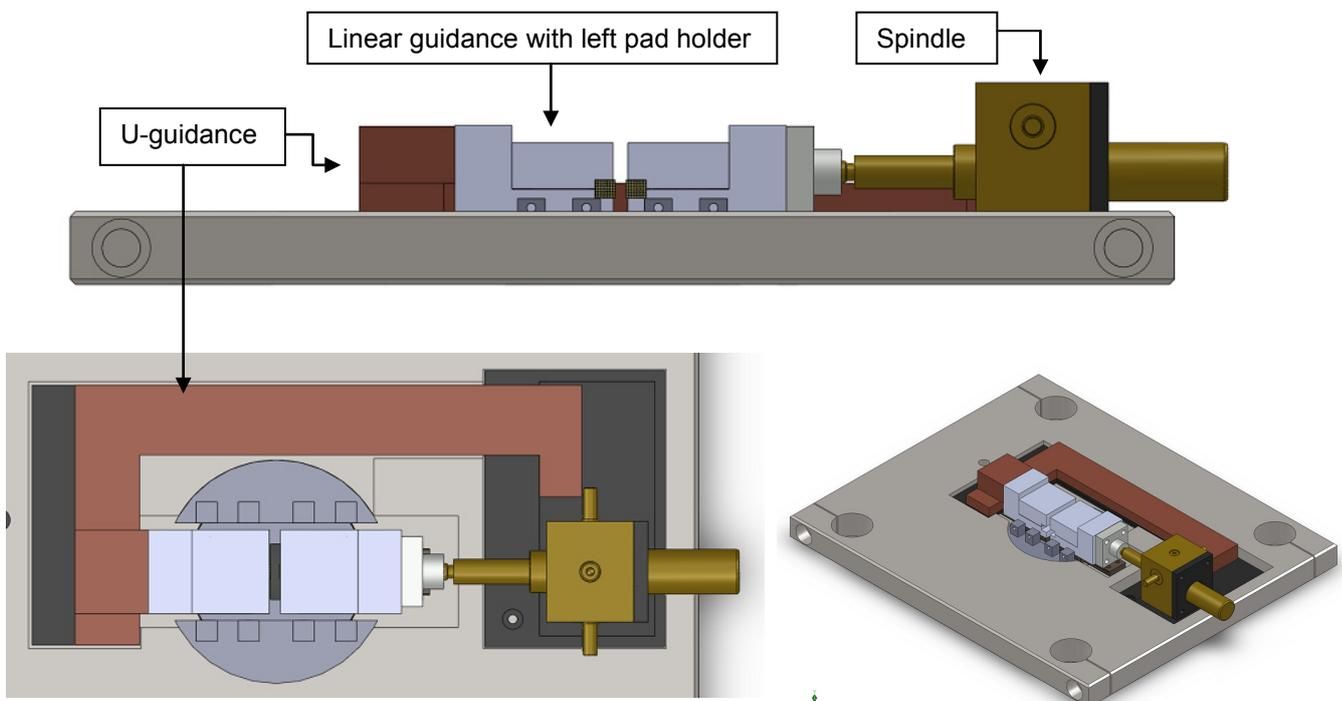
Figure 8: Concept 1: fretting fixture based on linear guides
