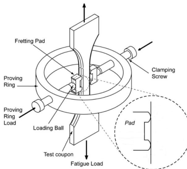
Figure 4: Proving ring test equipment
