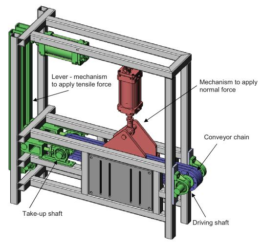
Figure 10: CAD-drawing of the designed test-rig
