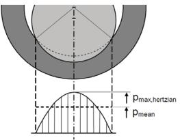
Figure 5: Hertzian pressure distribution in roller/bushing contact [10].
