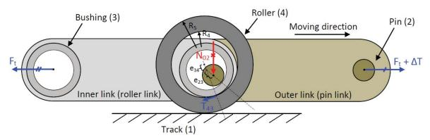
Figure 4: Section view of a roller conveyor chain with exaggerated clearances
