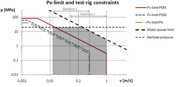
Figure 9: Pressure velocity limit of different polymers and test-rig limitations
