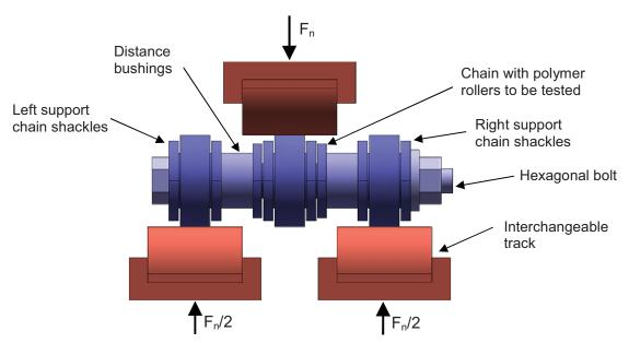
Figure 11: Loading principle of the chain
