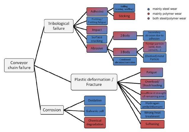
Figure 7: Wear mechanisms ocurring in conveyor chains
