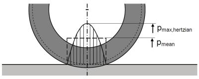
Figure 6: Hertzian pressure distribution in roller/track contact [10].
