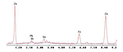
Figure 3. EDX analysis at crack tip [6]
