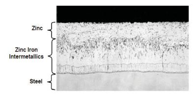
Figure 2. Typical galvanizing microstructure [2]
