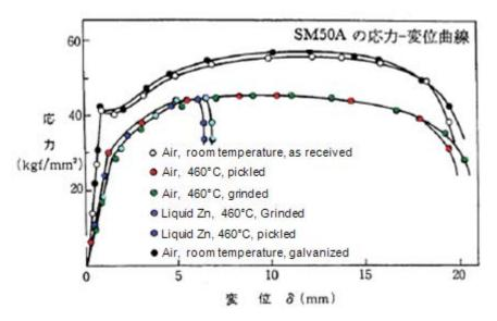
Figure 4. Stress/strain curves obtained from tensile tests [9]
