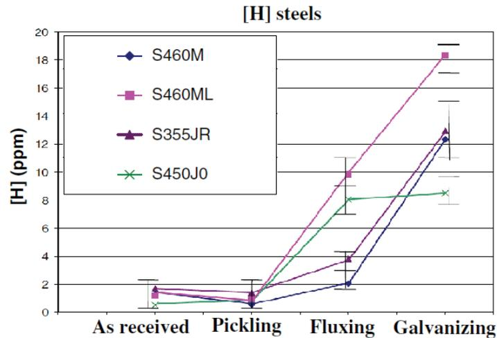
Figure 5. Evolution of hydrogen concentration on the steel surface[16]
