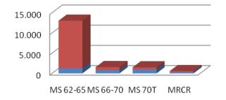
Graph 12. Number of maintenance tasks for the four series in the AM62-79 family. (period 01/07/2009 until 30/06/2010) Legend: Blue=planned maintenance and Red = unplanned maintenance
