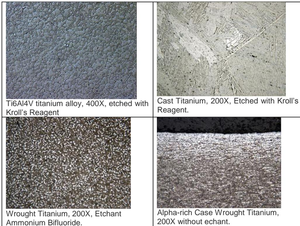
Figure 3. Microstructures of Titanium after polishing and etching [11]
