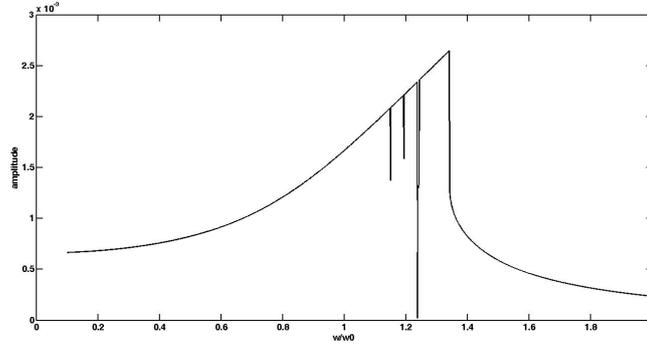
Figure 1. Classical harmonic balance method with  $N_h = 1$
