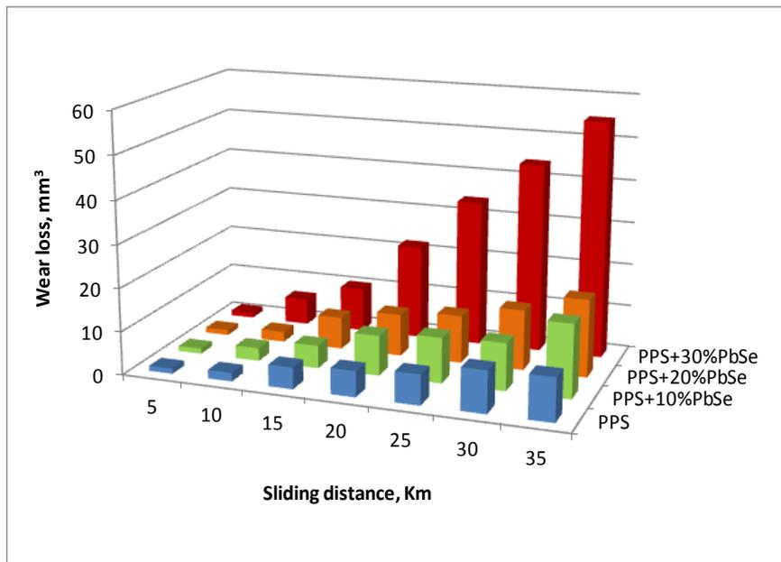
Figure 3. Results reported by Zhao and Bahadur of the wear loss of PPS filled with three difference proportions of PbSe with a test conditions: sliding distance speed 1.00 m/s, nominal pressure 0.65 MPa, counterface roughness 0.10  $\mu\text{m Ra}$ .
