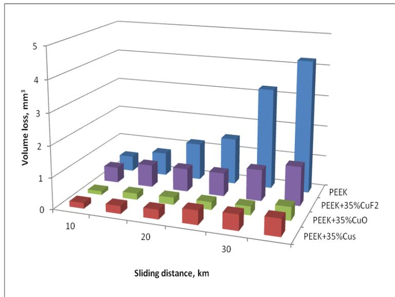
Figure 1. Results reported by Bahadur and Gong with the test conditions: sliding velocity 1.0 m/s, contact pressure 0.654 MPa, counterface roughness 0.11  $\mu\text{m Ra}$ .
