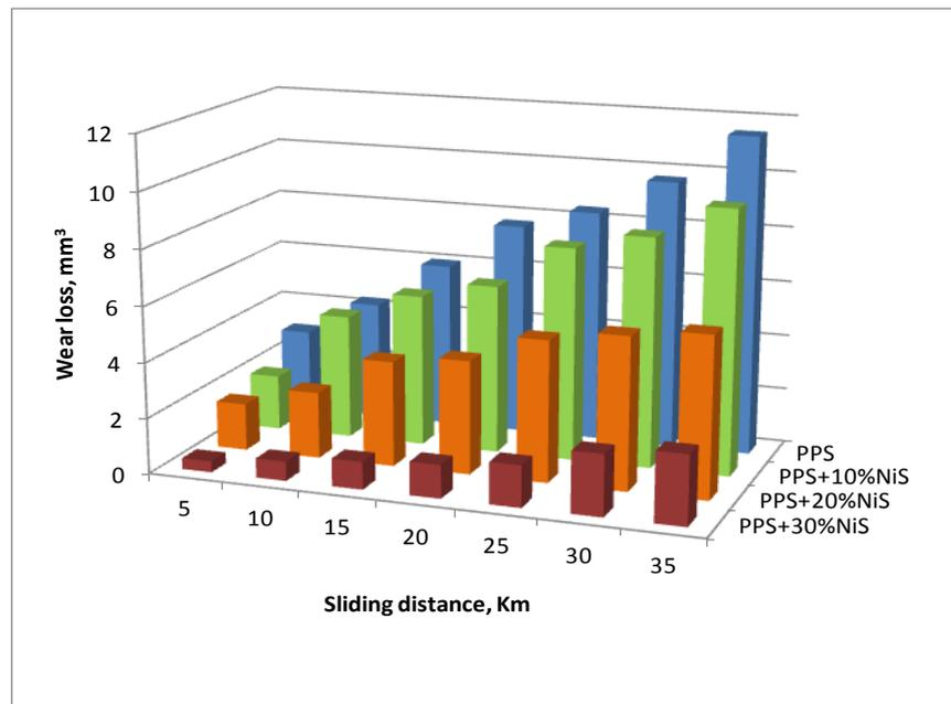
Figure 2. Results reported by Zhao and Bahadur of the wear loss of PPS filled with three different proportions of  $\text{NiS}$  with a test conditions: sliding distance speed 1.00 m/s, nominal pressure 0.65 MPa, counterface roughness  $0.10 \mu\text{m Ra}$
