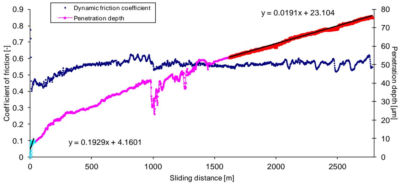
Figure 1. On-line monitoring of friction coefficient and penetration depth for SiC balls sliding against binderless WC flats with a contact pressure of 1.9 GPa and a speed of 0.3 m/s
