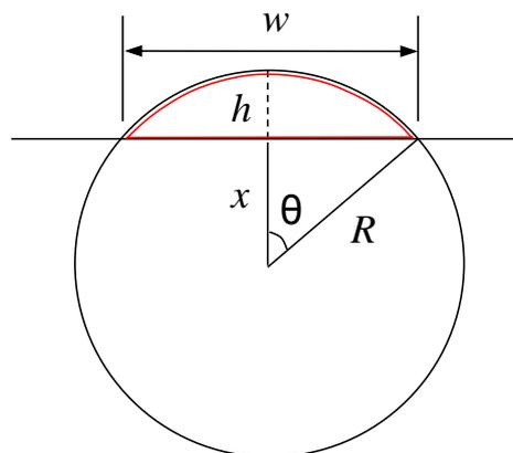
Figure 4. Geometrical analysis of the cross section of the ball, including the worn cap after the wear test.
