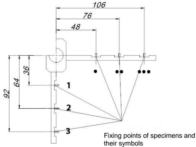
Figure 2. Specimens placed on different radiuses
