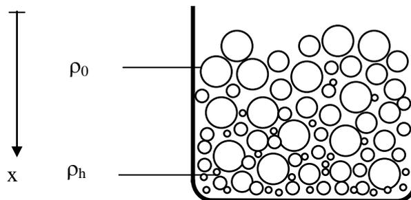
Figure 5. The changing of the abrasive medium aggregation-density (space filling, or "porosity") the lamination of grains (grain distribution) during measurings.
