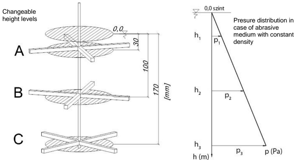
Figure 4. Changeable specimen-holder tool levels, and the pressure distribution changing linearly in case of abrasive medium with constant density.
