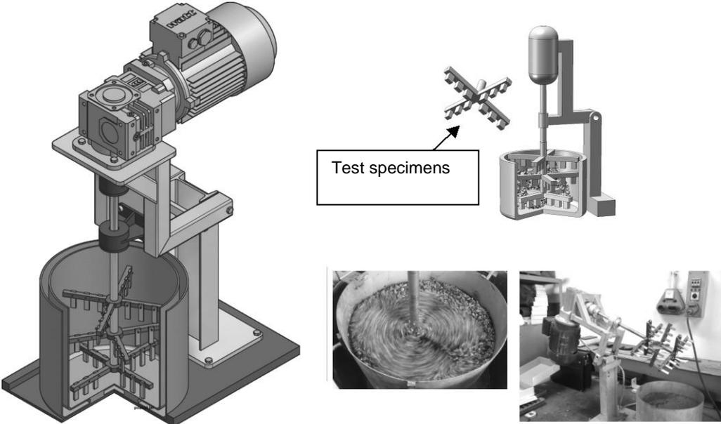
Figure 1. Modified “sand-slurry” module for abrasion measurements
