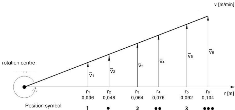
Figure 3. The positions of nests formed on the specimen-holders and speed vectors of the specimens at certain places in case of constant shaft revolution.
