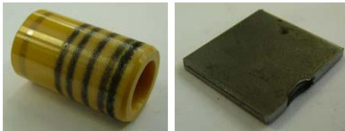
Figure 1. Frictional path formed on the ceramic surface and a worn steel specimen.
