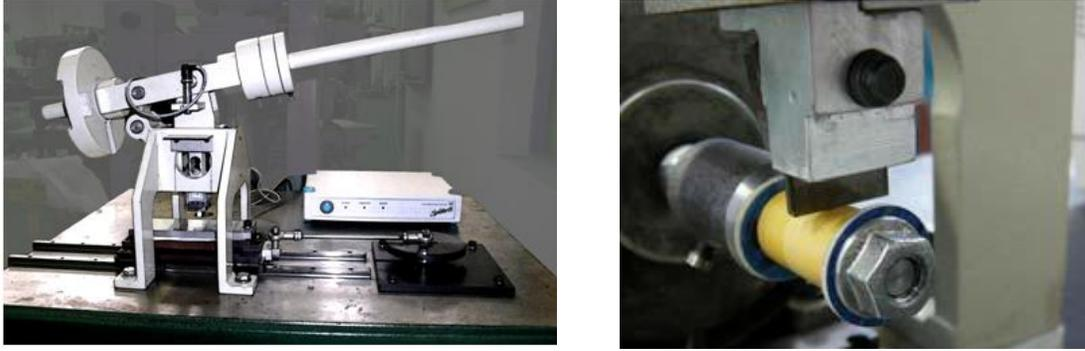
Figure 3. The basic equipment (Zsidai et al 2006; Lefánti et al 2011) and the clamped ceramic and steel specimens developed to the frictional test.
