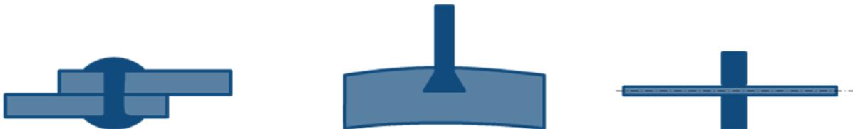
Figure 2. Overview of some applications where fretting fatigue has been reported.
