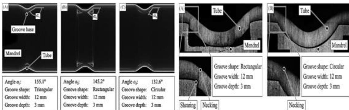
Figure 3. EMP crimping: resulting angle  $\alpha$  (left) and comparison of grooves (right) [8].
