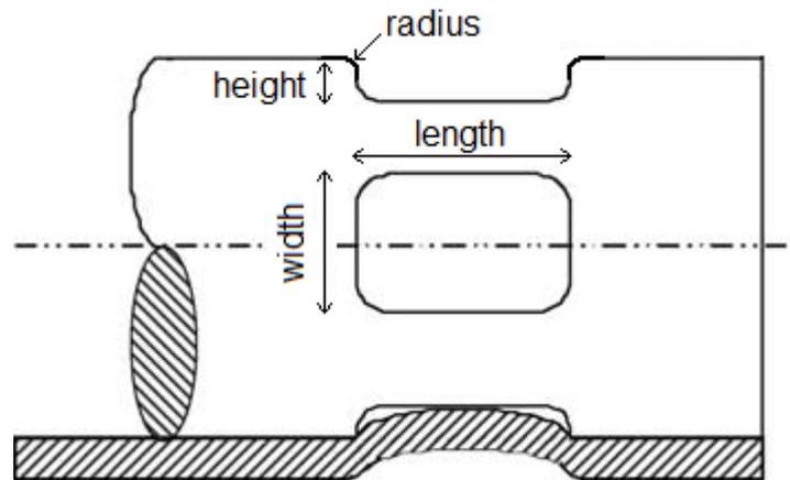
Figure 4. Main geometric design parameters of the used rectangular grooves [9].
