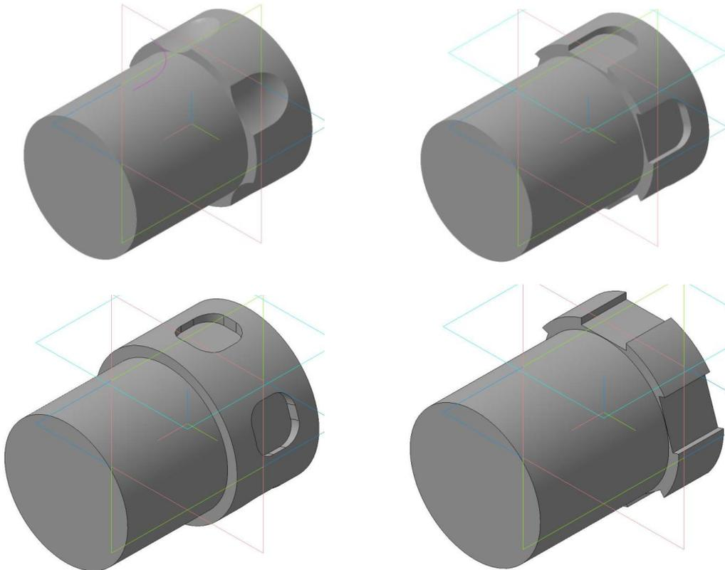
Figure 6. The 4 designs used in the preliminary experiments
