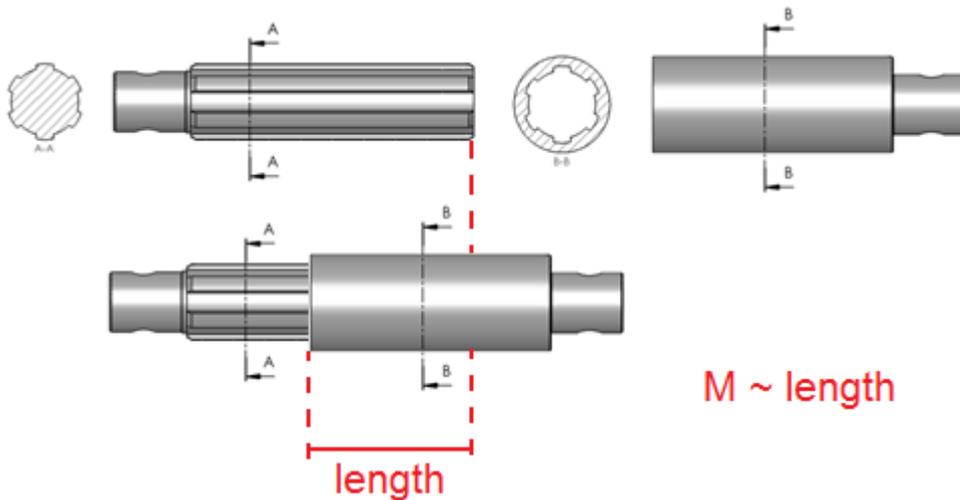
Figure 7. Spline coupling to illustrate the influence of groove length.
