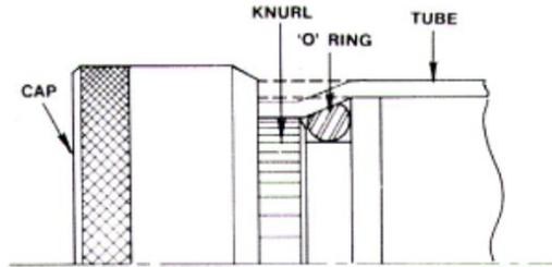
Figure 2 Suggestion for the use of an O-ring in EMP crimped joints [4]
