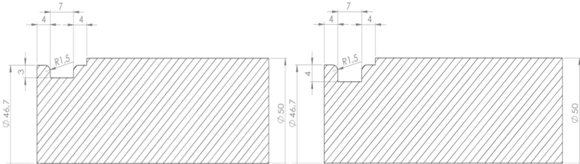
Figure 6 Design of the mandrels for the evaluation of O-rings.
