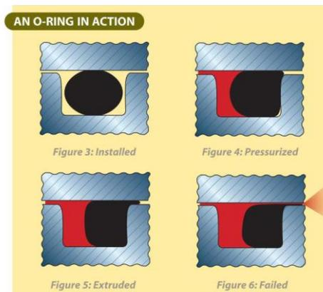
Figure 3 Working principle of an O-ring [7].
