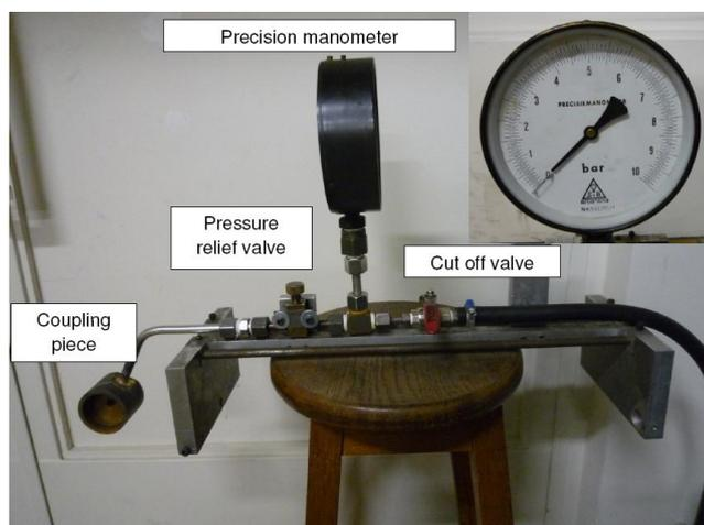
Figure 9 Air pressure test configuration [14]
