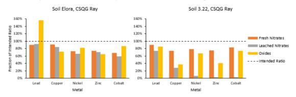
Figure 1: Difference in metal recovery due to soil type, leaching, and dose method.
