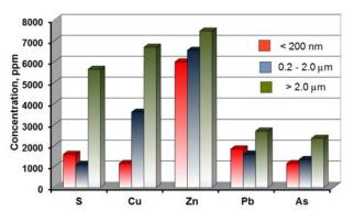
On the other hand, results of EDS microanalysis showed that a considerable part of dust microparticles are S, As, Cu, and Zn compounds, probably sulfides. These microparticles are of direct anthropogenic origin, emitted from copper smelter stack. Taking into account EDS data, higher concentrations of S, As, Cu, and Zn in rough fractions are quite logical.
