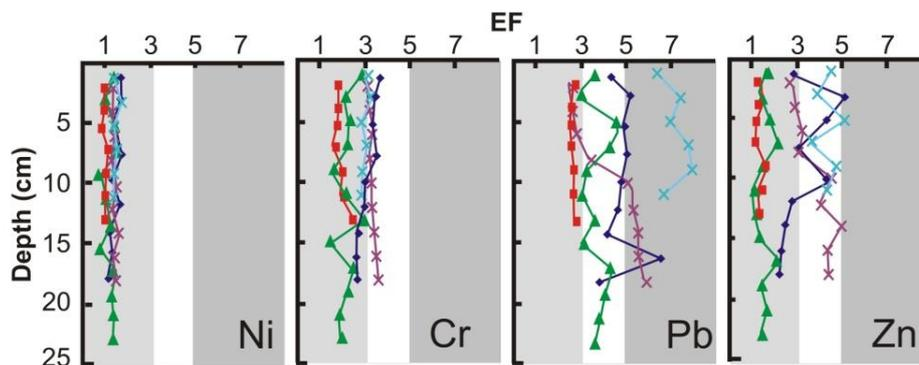
**Figure 1.** Enrichment factor (EF) values for Ni, Cr, Pb and Zn in five core samples from the Platier d'Oye. EF < 3 indicates minor enrichment, EF = 3-5 moderate enrichment, EF = 5-10 moderately severe enrichment.
