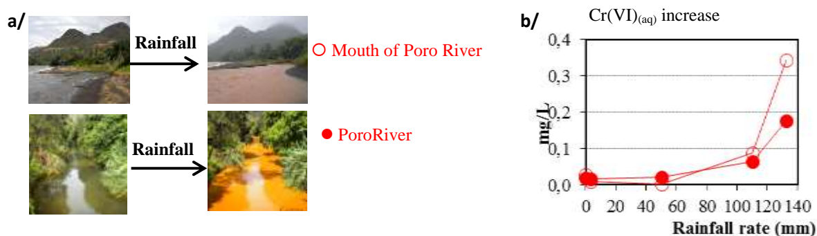
Figure 1: Opencast mines induce particulate matter runoff downstream (a) and dissolved Cr(VI) content increase (b)
