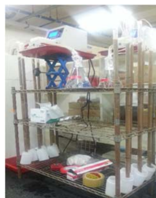
Figure 2. Column leaching system installation
