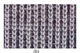
Figure 1. Right side of two fabric variants with 10 warp and 10 weft reinforcing yarns on the same scale: (a) Variant 1 (b) Variant 2
