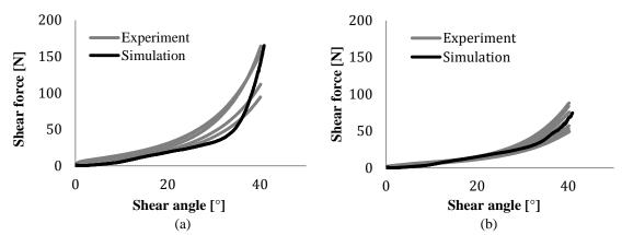
Figure 9. Comparison of shear force – shear angle curve between simulation and experiment of (a) Variant 1 and (b) Variant 2
