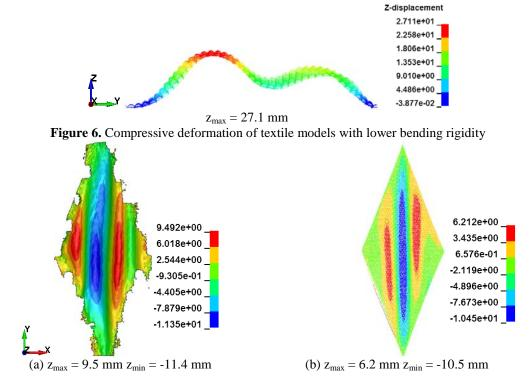
Figure 7. Optical comparison of the wrinkle size of fabrics variant 1 (a) Experiment (b) Simulation
