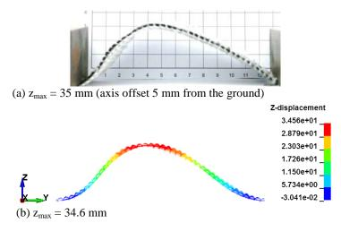
Figure 5. Compressive deformation of textile: (a) Real fabrics variant 1 (b) Equivalent model of variant 1
