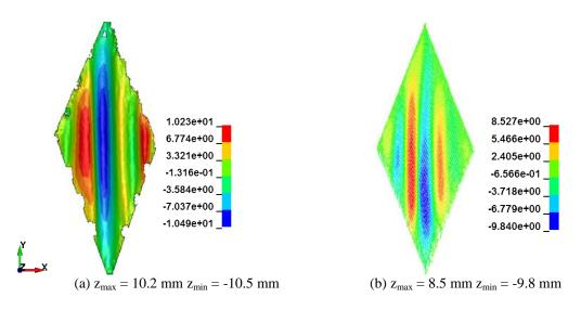
Figure 8. Optical comparison of the wrinkle size of fabrics variant 2 (a) Experiment (b) Simulation
