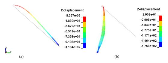
Figure 4. Simulation of cantilever test of textile: (a) correct bending rigidity (b) lower bending rigidity
