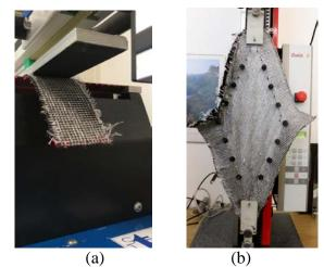
Figure 2. (a) Cantilever test machine (b) Tensile machine with picture frame 200 x 200mm
