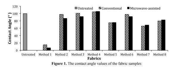
The contact angle will be less than  $90^{\circ}$  on a hydrophilic surface. If the surface is hydrophobic the contact angle will be greater than  $90^{\circ}$ . Untreated fabric had a fairly hydrophobic surface and showed a water contact of  $100^{\circ}$ .
