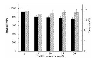
Figure 1. Tensile strength and elongation of PI fiber by NaOH treatment
