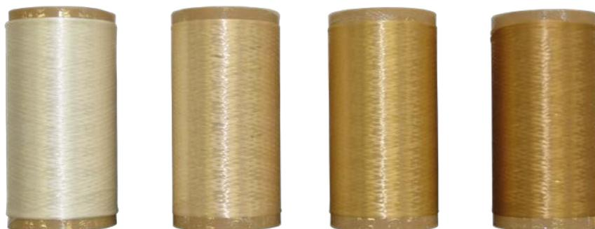
**Figure 2.** Wet spun PAN and PAN/lignin (5, 10 and 15 wt%) blend fibers
