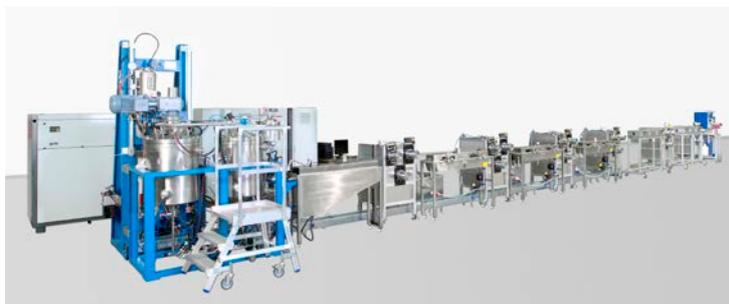
**Figure 1.** Wet-spinning pilot plant by Fourné Polymertechnik GmbH
