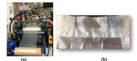
(a) (b) Figure 1. (a) flat die extrusion facility at University of Pisa (DICI) and (b) flat die extruded film based on plasticized PLA/PBAT
